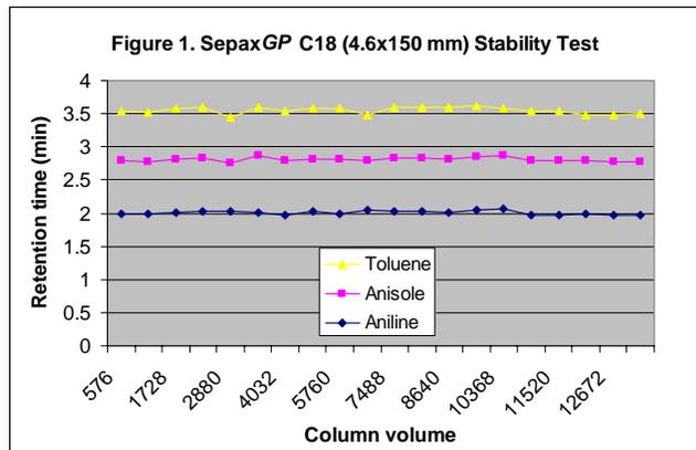
Such high stability allows SepaxGP-C18 extremely suitable for validation of various analytes. The unique mono-functional
