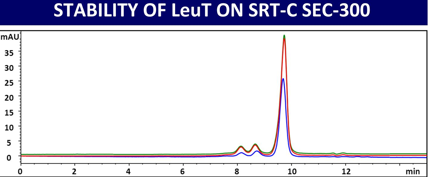
Injections of LeuT on SRT-C SEC-300 over the course of one month. The mobile phase was 20 mM Tris-HCl pH 7.0 with 190 mM NaCl, 10 mM KCl, and 40 mM OG. The flow rate was 1.0 mL/min. 10 µL of LeuT (1.0 mg/mL and blue trace is 0.5 mg/mL) was injected onto each column. Detection is at UV 280 nm.
