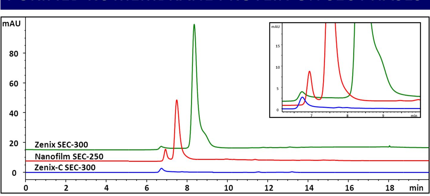
Analysis of purified bacterial photosynthetic reaction center (RC) membrane protein on three different size exclusion phases. The mobile phase was 10 mM Tris, pH 8.0 with 0.1% LDAO. The flow rate was 0.8 mL/min. 10  $\mu$ L of the membrane protein (1.0 mg/mL concentration) was injected onto each column. Detection is at UV 280 nm.
