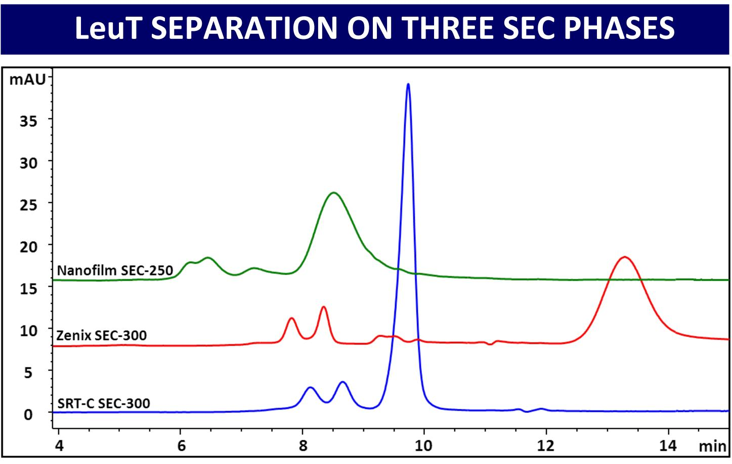
Analysis of the membrane protein LeuT on three different size exclusion phases. The mobile phase was 20 mM Tris-HCl pH 7.0 with 190 mM NaCl, 10 mM KCl, and 40 mM OG. The flow rate was 1.0 mL/min. 10  $\mu$ L of the membrane protein (1.0 mg/mL concentration) was injected onto each column. Detection is at UV 280 nm.
