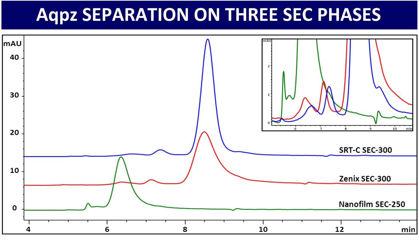
Analysis of the membrane protein Aqpz on three different size exclusion phases. The mobile phase was 20 mM Tris-HCl pH 7.0 with 190 mM NaCl, 10 mM KCl, and 40 mM OG. The flow rate was 1.0 mL/min. 2 µL of the membrane protein (6.0 mg/mL concentration) was injected onto each column. Detection is at UV 280 nm.
