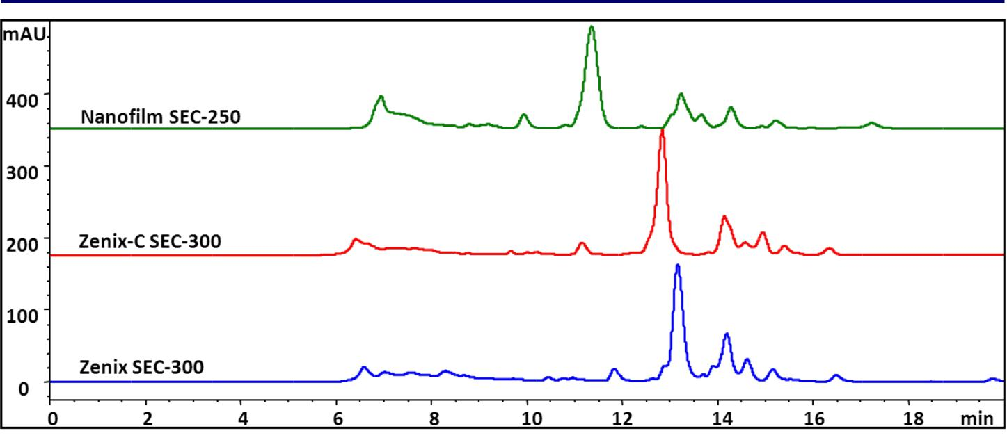
Analysis of rhodo bacteria lysate on three different size exclusion phases. The mobile phase was 10 mM Tris, pH 8.0 with 0.1% LDAO. The flow rate was 0.8 mL/min. 5  $\mu$ L of the membrane protein was injected onto each column. Detection is at UV 280 nm.
