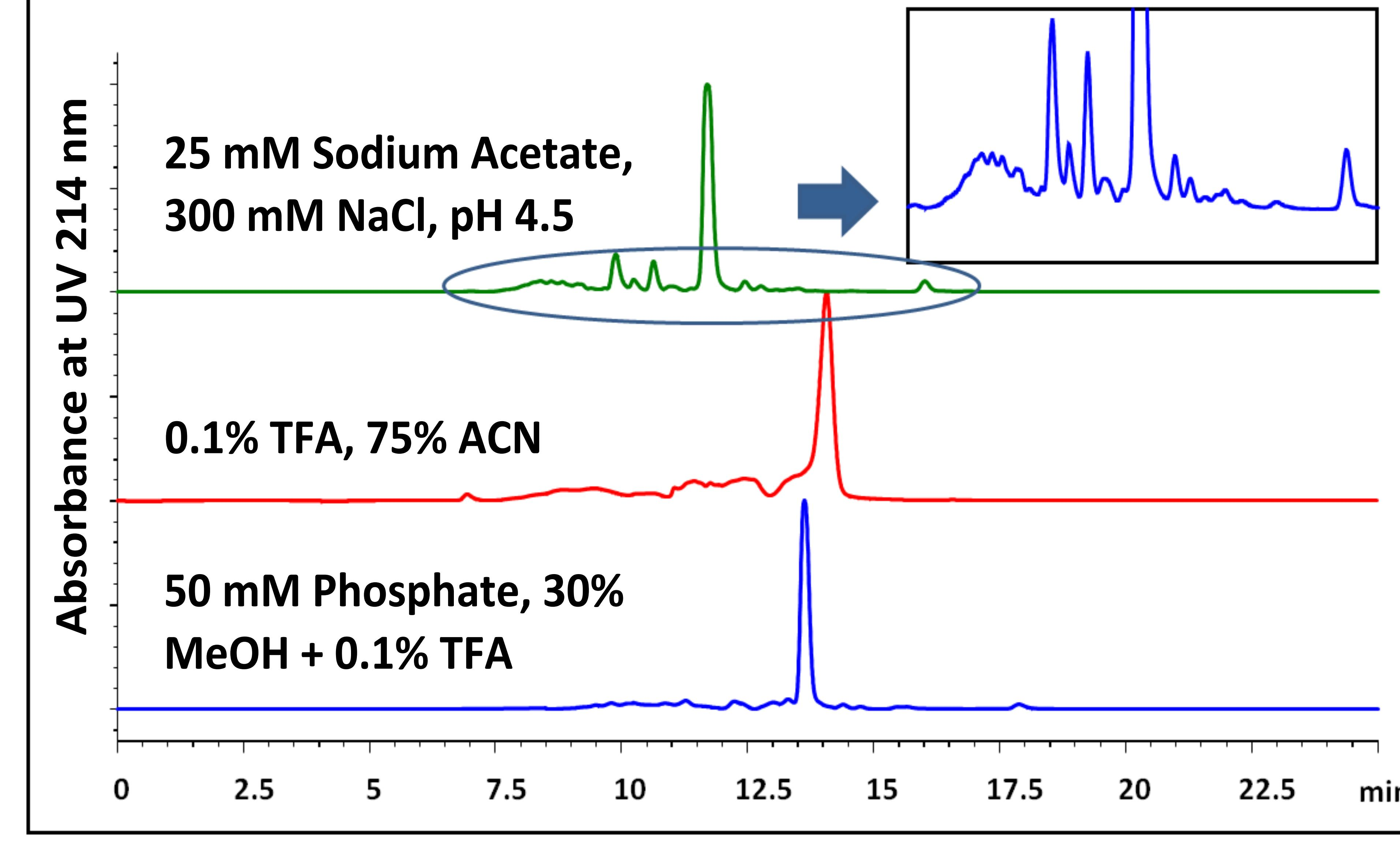
For complex E. coli tryptic digest, a mobile phase of 25 mM sodium acetate/300 mM NaCl gave the best separation. The bottom chromatogram was run with 50 mM phosphate/30% MeOH/0.1% TFA. The middle one was run with 0.1% TFA/75% ACN. The top chromatogram represents the best degree of peptide separation and was run with 25 mM sodium acetate/300 mM NaCl, pH 4.5.
