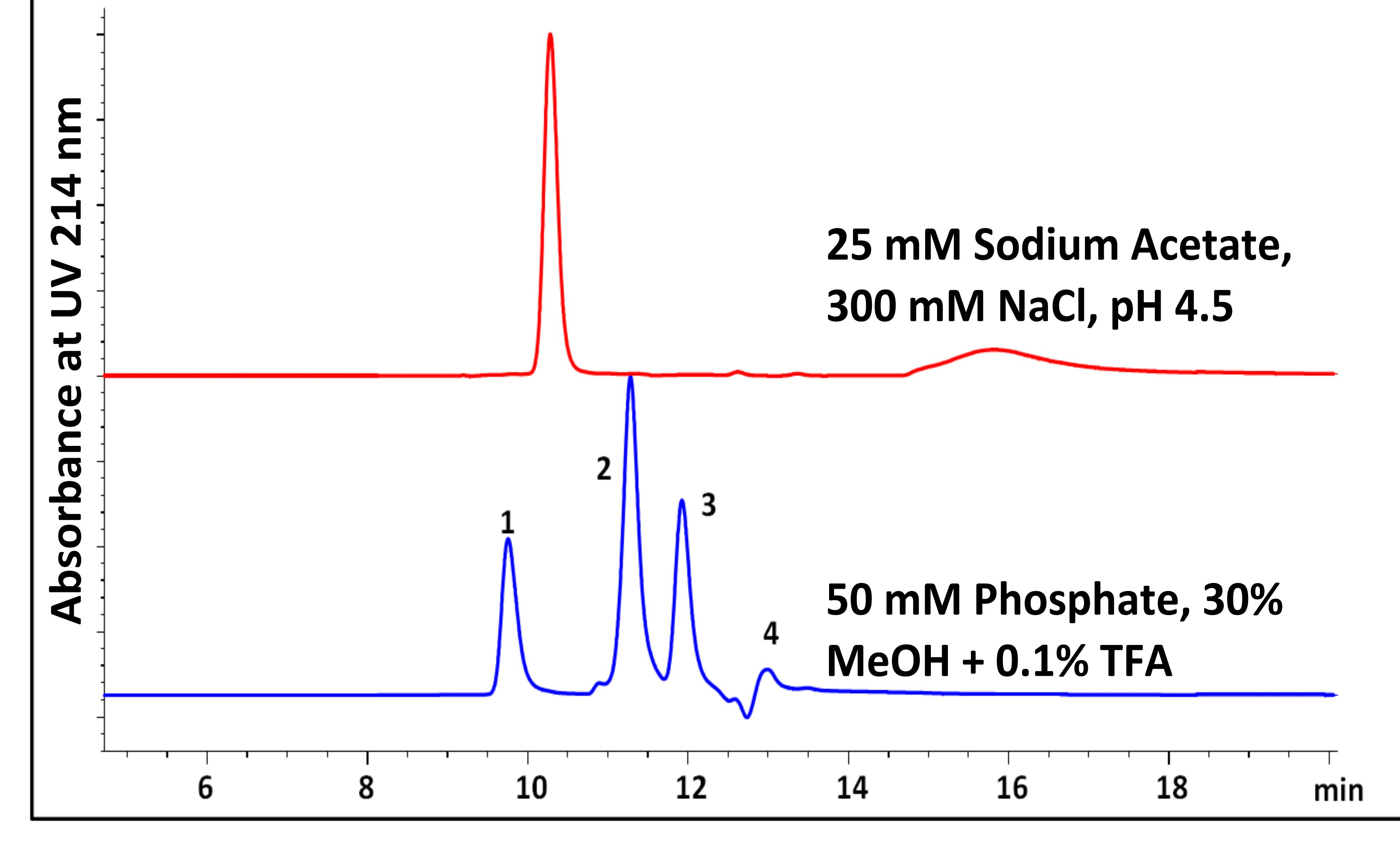
Peak elution order: 1. Insulin, 2. Bradykinin, 3. Angiotensin I, 4. Glucagon. The flow rate was 0.8 mL/min. The top chromatogram was run with the mobile phase of 25 mM sodium acetate and 300 mM NaCl, pH 4.5. The bottom one was run with the mobile phase 50 mM Phosphate with 30% MeOH and 0.1% TFA.
