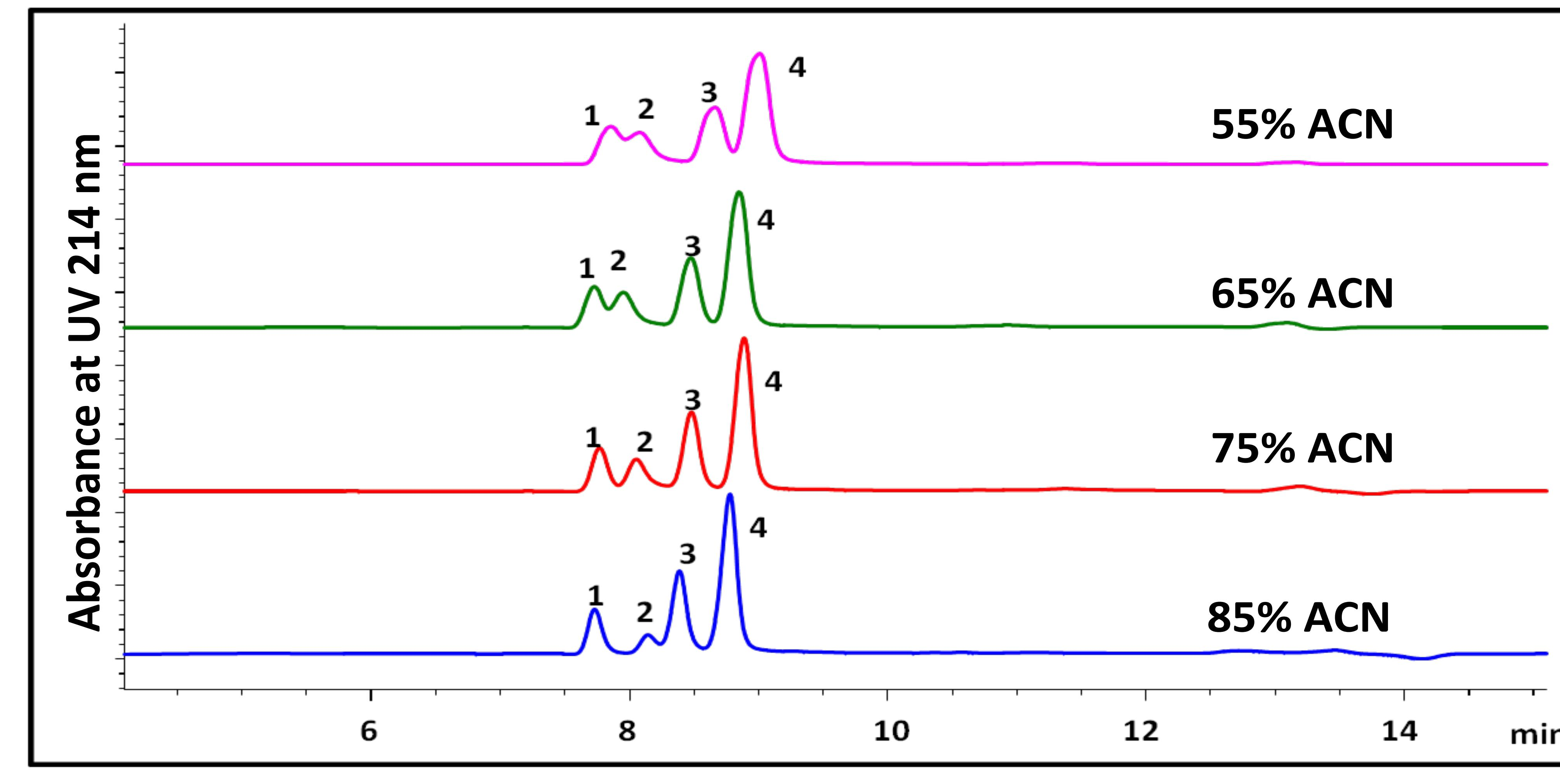
Effect of mobile phase acetonitrile concentration on the separation of the four peptide mixtures (Peak 1 Insulin, Peak 2 Glucagon, Peak 3 Angiotensin I, Peak 4 Bradykinin). The mobile phases contained 0.1% TFA with the indicated percentage of acetonitrile. The flow rate was 0.8 mL/min. 5  $\mu$ L of the peptide mixture (0.5 mg/mL concentration for each peptide) was injected.
