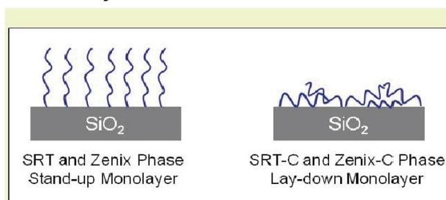
Figure 1. Phase structure difference: a monolayer stands up on the silica surface for Zenix and SRT, and a monolayer lays down on the silica surface for Zenix-C and SRT-C.
