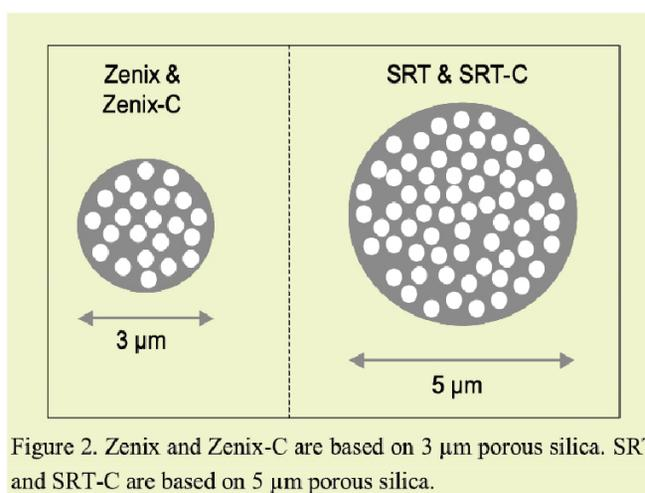
Figure 2. Zenix and Zenix-C are based on 3 μm porous silica. SRT and SRT-C are based on 5 μm porous silica.
