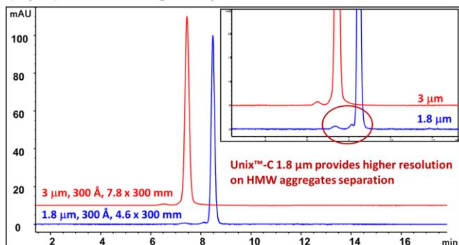
**Column:** Unix™-C SEC-300 (1.8 μm, 300 Å, 4.6 x 300 mm)
