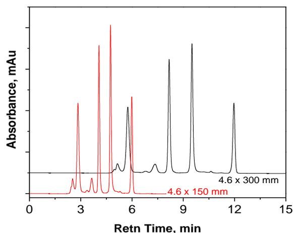
**Column:** Unix™-C SEC-300 (1.8 μm, 300 Å, 4.6 x 150 mm)
