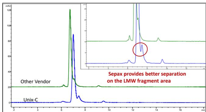
**Column:** Unix™-C SEC-300 (1.8 μm, 300 Å, 4.6 x 300 mm)
