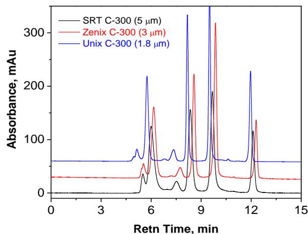
**Column:** Unix™-C SEC-300 (1.8 μm, 300 Å, 4.6 x 300 mm)
