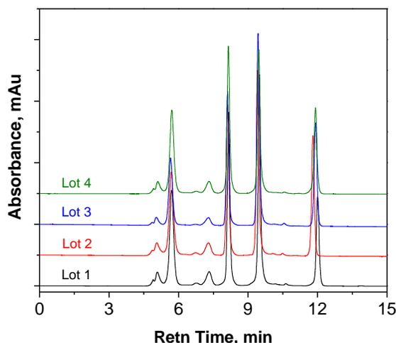
**Column:** Unix™-C SEC-300 (1.8 μm, 300 Å, 4.6 x 300 mm)
