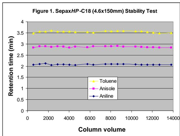
Such high stability allows SepaxHP-C18 extremely suitable for validation of various analytes. The unique mono-functional bonding chemistry for SepaxHP-C18 avoids the formation of multiple C18 layers. Such uniform stationary phase allows the separation to achieve high selectivity and high efficiency. A typical test chromatogram for quality control is shown in Figure 2 for a 4.6x150mm SepaxHP-C18 column.
