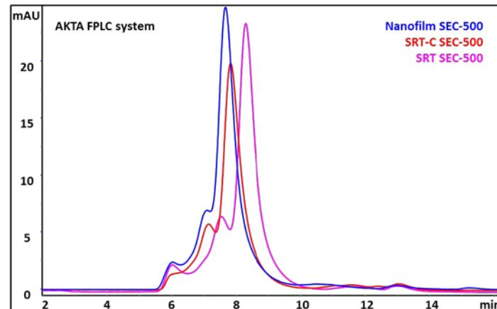
**SRT SEC-500 best separated the aggregates of Ferritin in the presence of detergent.**
