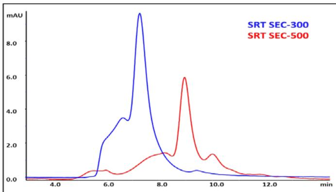
**SRT showed better separation and larger pore size 500 Å may help with separation of aggregates and monomer; however the recovery may be lower.**
