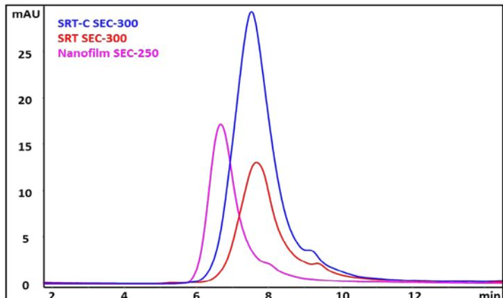
SRT-C gives the best separation with less secondary interaction, baseline separation with the high molecular weight proteins.
